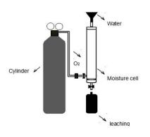
sample was subjected to the environmental conditions of the site. A kinetic test was carried out in two cycles, lasting 7 and 6 days each, using a moisture cell according to Sobek, Schuller, Freeman and Smith (1978). Using this test also information was obtained on the resulting acidic conditions and the quality of the leachate produced.
