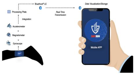
FIGURE 5 Deployment diagram of IMU system.
