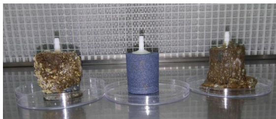
Fig. 2. Air diffusers at the end of removal test No. 2. From left to right: Aspergillus sp., control, and Penicillium dipodomycicola strain IIF7SW-F4.
