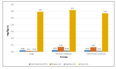
Figure 3. Total phosphorus ( $P_2O_5$ ), potassium (KO), magnesium (Mg) and calcium percentage for the sludge coming from drying bed, the enzymatic composting and non-enzymatic composting. (2012)
