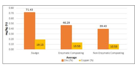
considered a non-toxic substrate. For the sludge coming from the drying bed, the concentration (mg/L) of Zinc and Cupper are 71.43 and 19.13 respectively, for the enzymatic composting are 46.29 and 13.53 respectively, and for the non-enzymatic composting are 39.43 mg/L Zn and 10.53 mg/L Cu.
